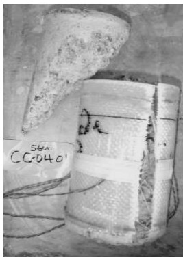
Figure 2: Failure of concrete-filled GFRP tubes
