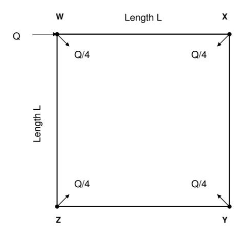
Fig. 4. Simple loop example with demand allocated equally to nodes
