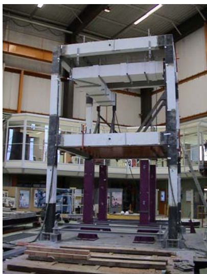
Fig. 4 FRP strengthened frame
