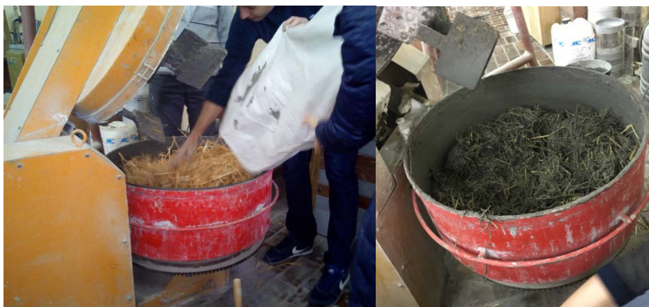
Figure 1. Students of Faculty of Civil Engineering in Subotica, on the subject Traditional materials processing wheat straw by treating in a mixer with impregnating materials to achieve strength after the compressing phase (straw, cement, lime, pucolic powder, water, chemical impregnation agents)
