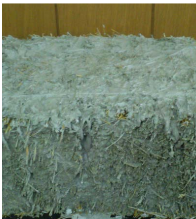
Figure 3. Surface treatment and impregnation of straw-bale, performed by students of the Faculty of Civil Engineering in Subotica on the subject Traditional Materials
