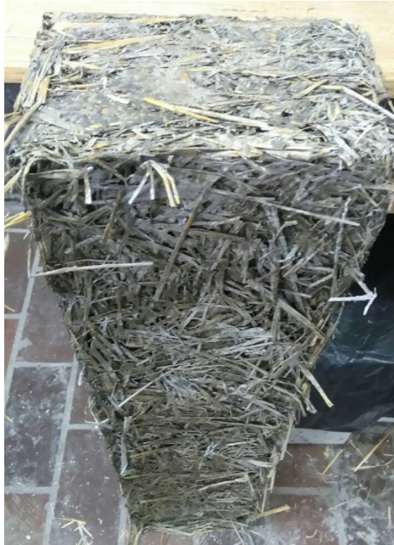
Figure 4. . Pre-treatment and impregnation of straw as a fibrous aggregate in the mixers and afterwards, pressing into the masonry elements were made by students of the Faculty of Civil Engineering in Subotica on Traditional Materials
