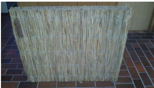
Figure 5. Wall panels made of cane
