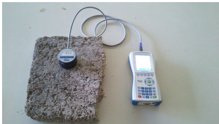
Figure 8. Measuring of the heat conductivity on the hemp-crete
