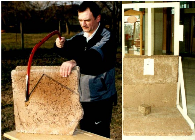
Figure 9. Hemp-concrete elements ready to be used for separating walls and for lightweight and warm screeds
