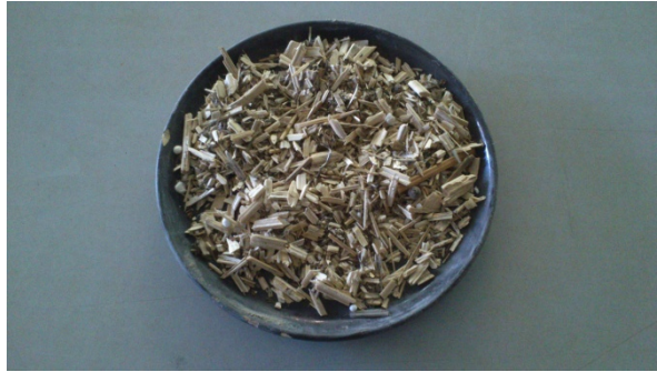
Figure 7. Shiv granulate obtained by grinding hemp stems
