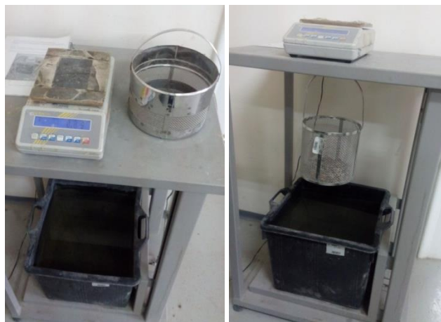
Figure 1 – Apparatus for absorption measurement of aggregate fraction II (left) and III (right)
