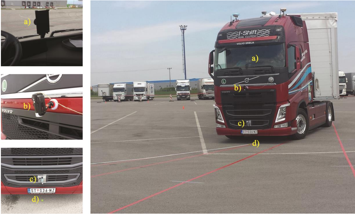
Fig. 4. Volvo FH 500 performing a 120° turning maneuver: (a) tablet computer, (b) high-resolution action camera, (c) laser designator mounted on Volvo front bumper, and (d) green laser beam.
