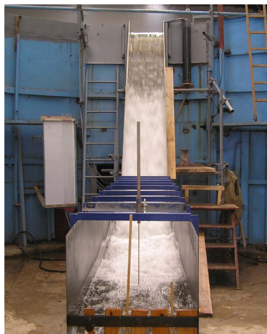
Figure 1. Scale model of the section of the weir with the stepped spillway of the Bogovina dam [14, 20]
