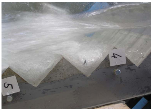
Figure 5. Air entrainment at the stepped spillway obtained by: a) scale-model, b) numerical model. The recirculating flow in the triangular cavity, formed by the steps, was observed on the scale model as well as the air entrained in the cavity. The numerical model was able to reproduce the recirculating flow pattern in the cavity (see the streamlines). Modelling of air water mixing was restricted to the free surface zone, but was not reproduced within the cavity itself.
