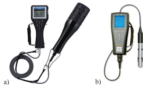
Slika 2. Multiparametarska sonda HORIBA U54G (a) i sonda za temperaturu i rastvoreni kiseonik YSI ProODO Figure 2. Multiparameter probe HORIBA U54G (a) and two-parameter (temperature and DO) probe YSI ProODO with optical dissolved oxygen sensor
