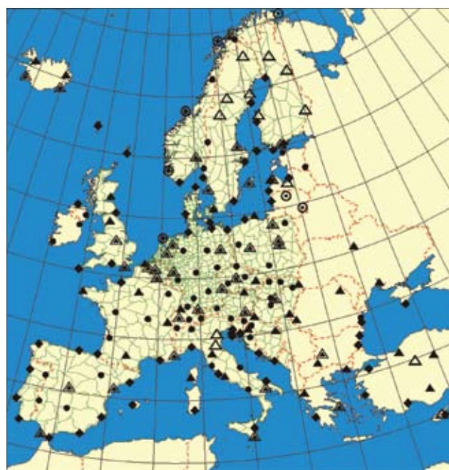
▲ EUREF sites ▲ GPS permanent stations - EUREF △ GPS permanent stations • UELN & UPLN nodal points ⊙ GPS permanent stations - nodal points ◆ Tide gauge sites ⊕ GPS permanent stations - tide gauge ~ UELN lines
