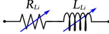
Figure III-11 Equivalent electrical diagram for the lift force applied to a blade element.
