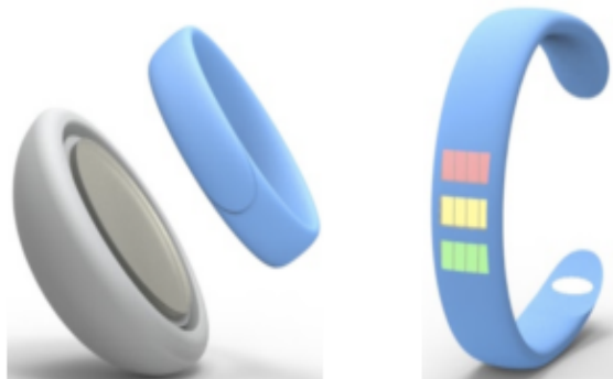
Figure 1: AwareMe. Haptic feedback is provided to the speaker using a wristband (Bubel et al., 2016).
