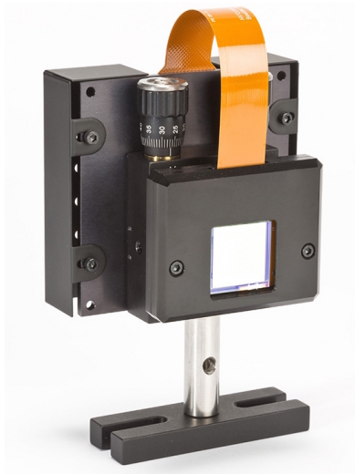
Figure 1.5: Spatial light modulator (SLM) . SLMs are computer-controlled devices used in experimental optics to generate arbitrary intensity, phase and polarisation patterns. Image from [54].
