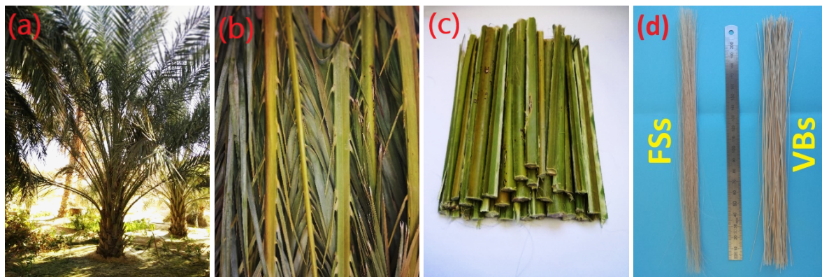
Figure 1. Photographs of (a) date palm tree, (b) date palm rachis and leaflets, (c) cut rachis, and (d) vascular bundles (VBs) and fiber strands (FSs).
