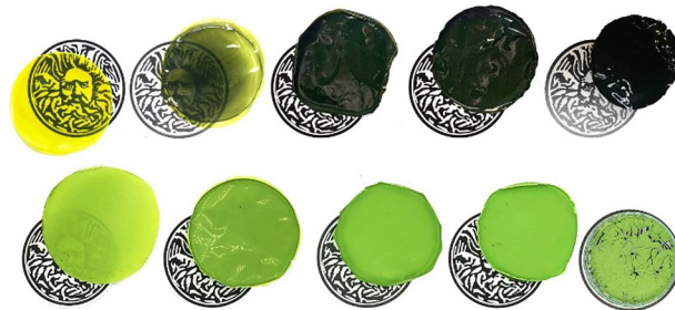
Fig. 2 Images of 6 cm diameter films, placed above the logo of the University of Bath to demonstrate varying transparency. Top row—left to right: PIM-1/AX21 composites with AX21 weight concentration at 0% (A0), 10% (A10), 20% (A20), 40% (A40) and 60% (A60). Bottom row—left to right: PIM-1/MIL-101 composites with MIL-101 weight concentration at 10% (M10), 20% (M20), 30% (M30), 40% (M40), and 50% (M50)
