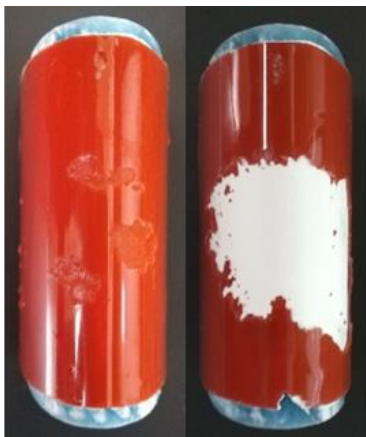
Figure 14. Coating samples after 20 minutes (left) and 35 minutes (right) in the ETC test rig.
