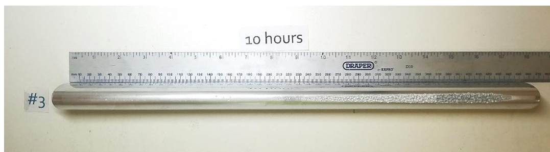
Figure 11. An aluminium sample after 10 hours in the ORE Catapult test rig at a rotational velocity of 1250 rpm.
