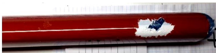
Figure 15. Coating sample after 16 hours in the ORE Catapult test rig.
