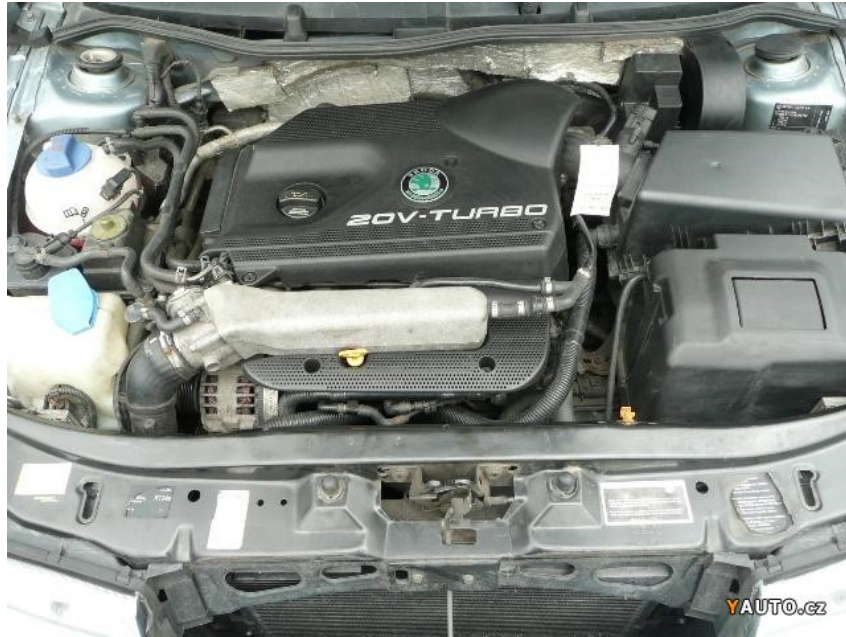
Figure 6: Skoda Octavia 1 Engine 1.8T 20V 110kW at 5700 rpm [12]
