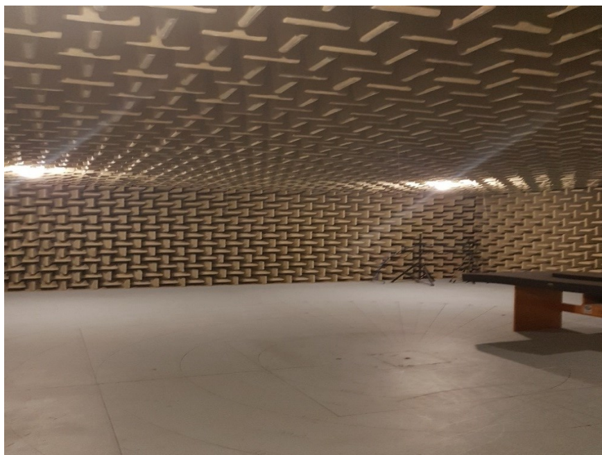
Figure 6.5 - Photograph from measurements taken in the semi-anechoic room of VŠB-TUO
