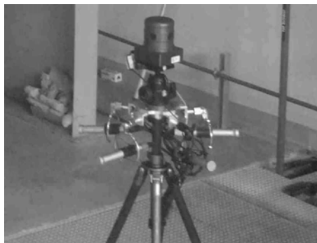
Figure 5.15: The Point Grey high resolution “Ladybug” 360° panoramic video camera (on top) to which our colleague Antoine Cordelois added a panoramic sound capture system (array of 5 microphones below).
