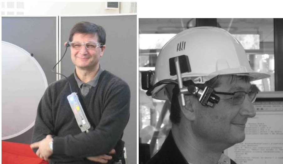
Figure 5.2: two versions of the SubCam: office work (left); plant version (right).
