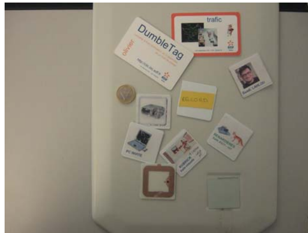
Figure 5.22: RFID ServiceTags on a reader (on the left notice the 1€coin for scale).
