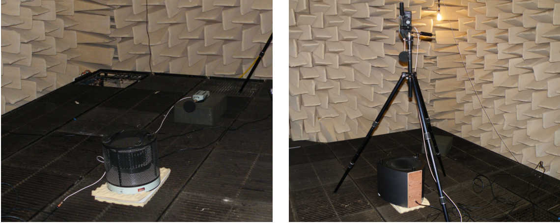
Figure 4.2: Directivity measurements in the anechoic chamber using the reference source (left) and subwoofer (right).
