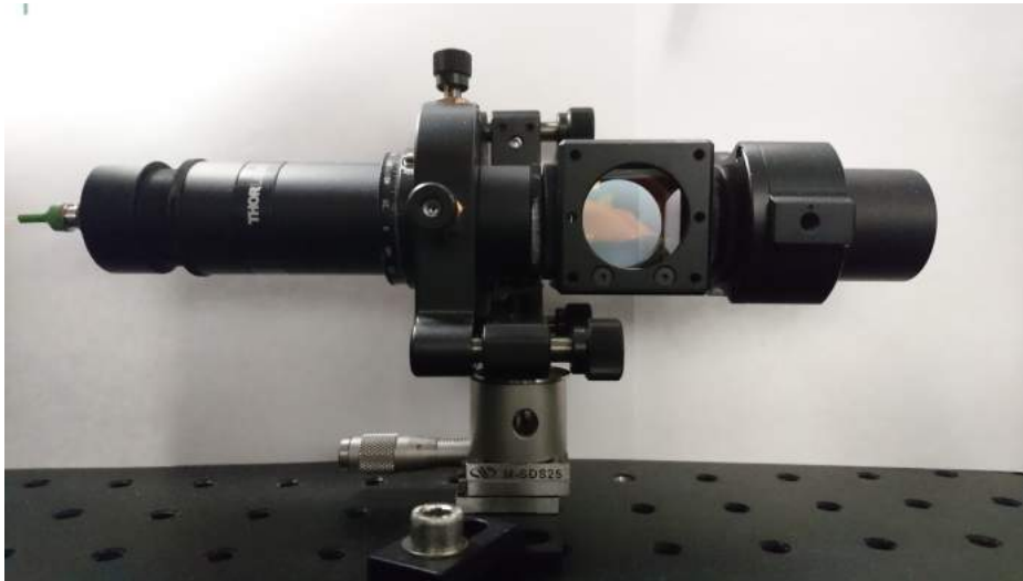
Fig. 5.20 An image of the newly designed outcoupler used to create a focused beam to act as a waveguide for atoms in the BEC.
