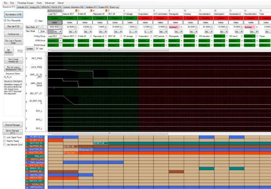
Fig. 3.12 Typical screenshot of a Cicero sequence. Analogue outputs appear in the middle of the image, each separate output is independently controlled with a range of voltages of \pm 10 V. Digital outputs are below and controlled with an on/ off toggle switch providing +5 or 0 V respectively. The horizontal axis represents increasing time in the sequence.
