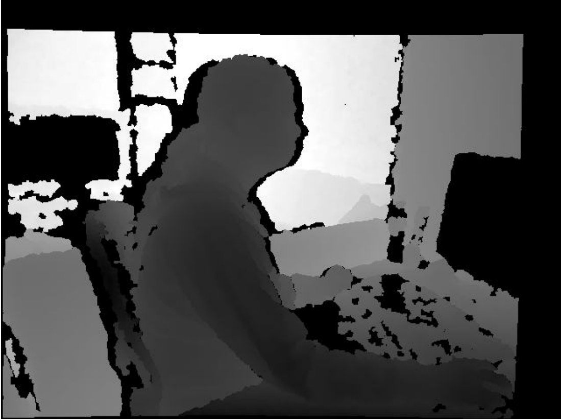
Figure 3.1: Depth map obtained from Kinect
