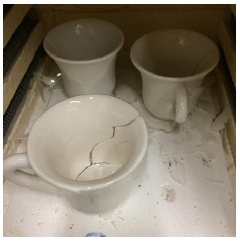
Fig. 3.24 'Making Of' *Kahvehane Kongresspark* (2016). Kütahya ceramic ware cracked in kiln due to glaze incompatibility.
