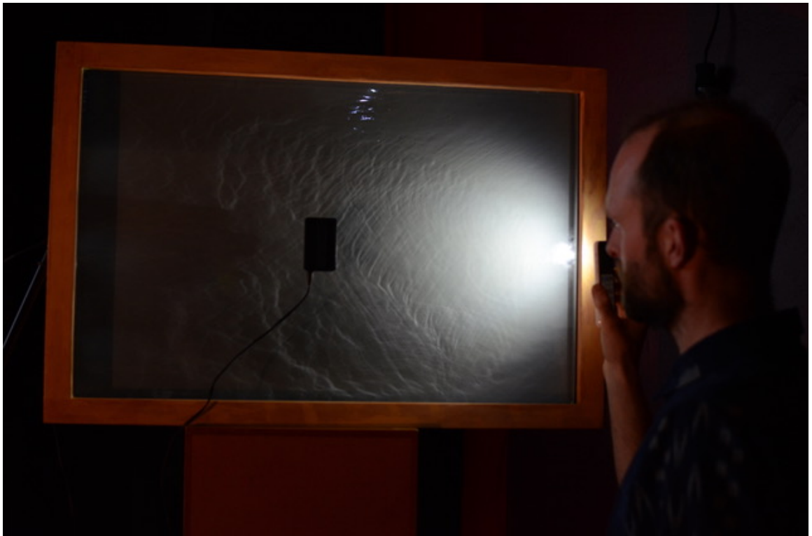
Figure 14: Resonant-window in its first formation, mounted in a self-built resonant box.
