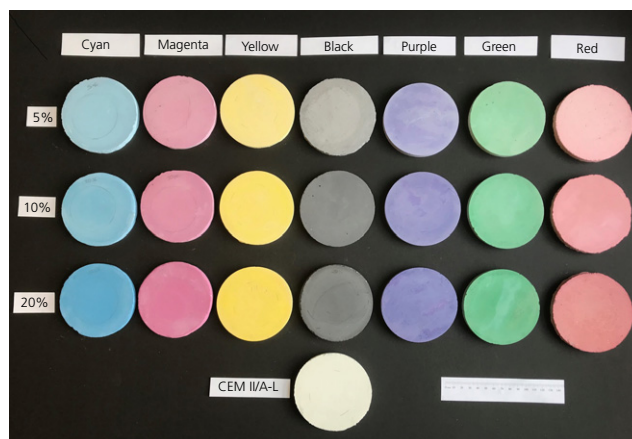
Figure 1. Paste specimens produced for the colour development study showing primary colours (cyan, magenta, yellow), secondary colours (purple, green, red), black, and control white (CEM II/A-L). A full-colour version of this figure can be found on the ICE Virtual Library ( www.icevirtuallibrary.com )
