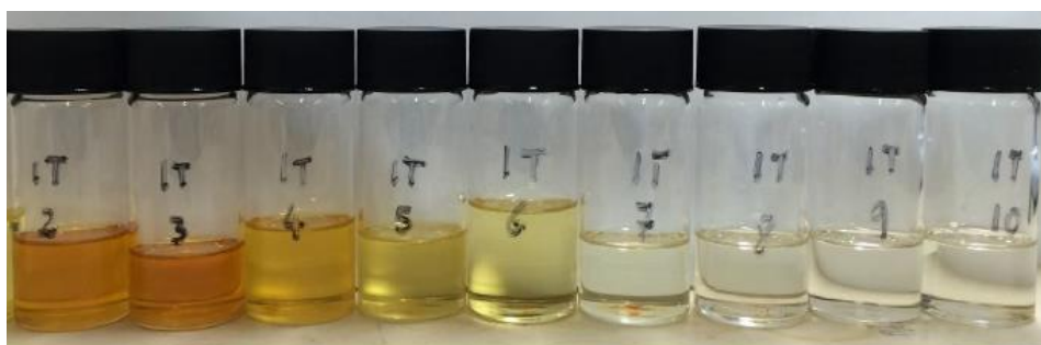
Figure S3-5. Washings to remove unattached surface units from 3@SiO_2@Fe_3O_4 (NP1).
