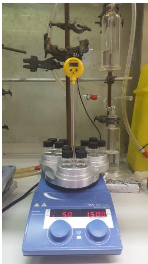
Figure S4-1. Multiwell heating block and stirrer hotplate apparatus with a thermometer.
