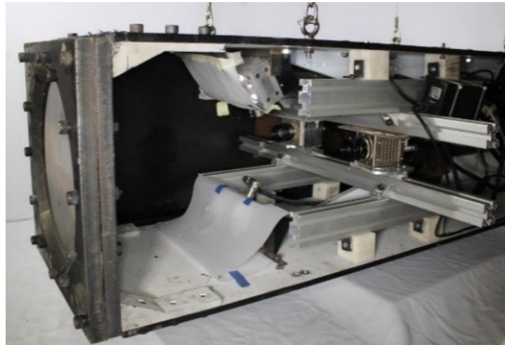
Figure 3-8- Photograph showing the inside of the modified, DIC pendulum, set up for filming the rear surface of the plates
