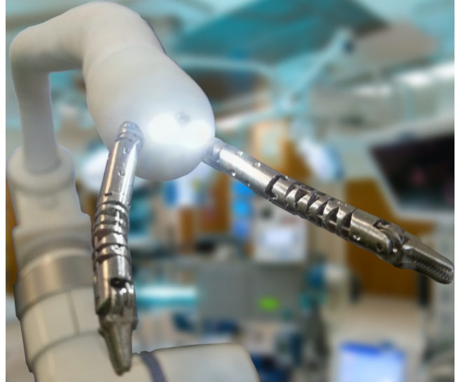
Fig. 1: Picture of the i 2 Snake (Intuitive Imaging Sensing Navigated and Kinetically Enhanced robot) prototype. The i 2 Snake is a robotic platform with a flexible body and equipped with vision, lighting and two robotic tools.
