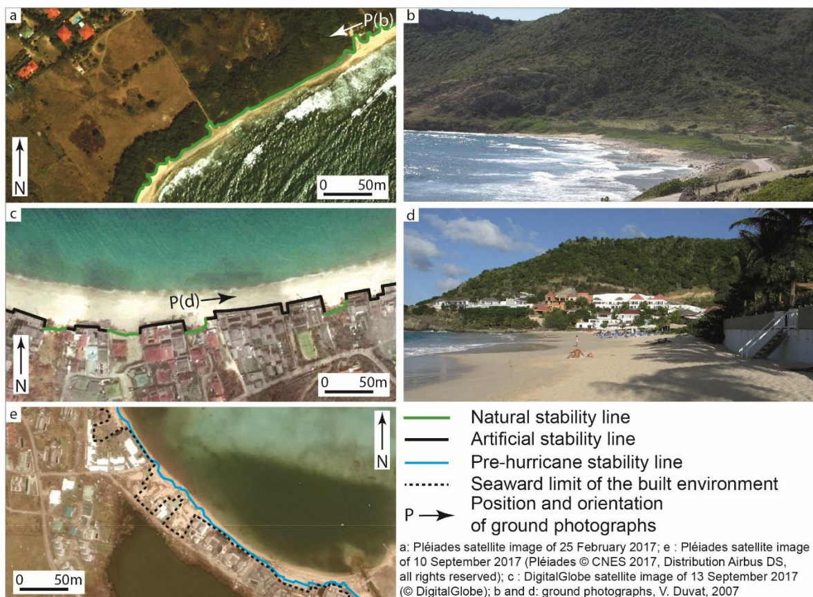
Fig. 6. Indicators used in this study to assess the contribution of longitudinal human constructions to beach response. (a) illustrates pre-hurricane ‘natural’ stability line. In this case, no human-built structure was present, as shown on photograph (b) (Grand Fond). (c) shows the alternation of artificial and natural stability line sections in
