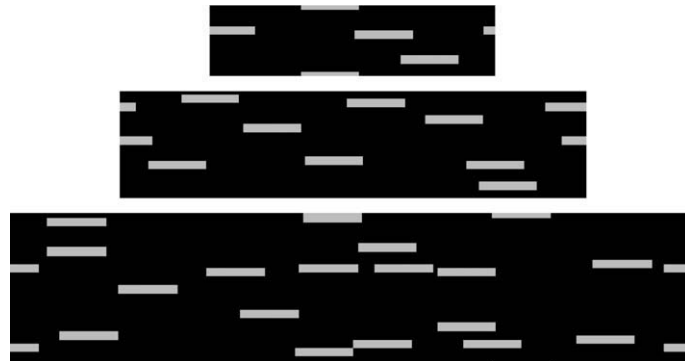
Fig. 12. Example of four periodic volumes, composed of 4, 10 and 20 inclusions, with f_v = 10\% .
