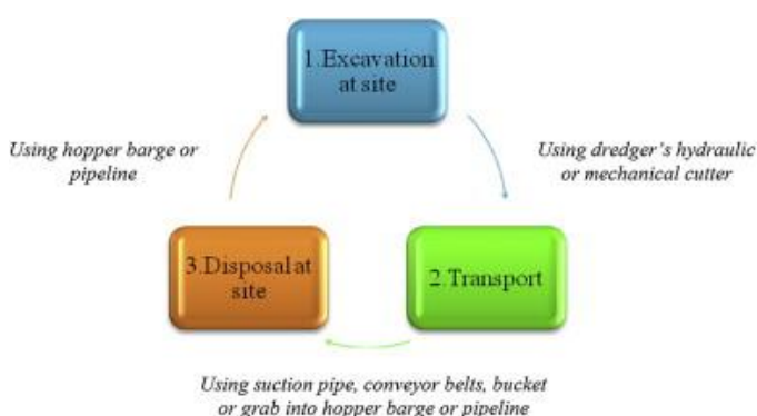
Fig. 1. Stages of dredging (Highley et al., 2007, Verbeek, 1984).
