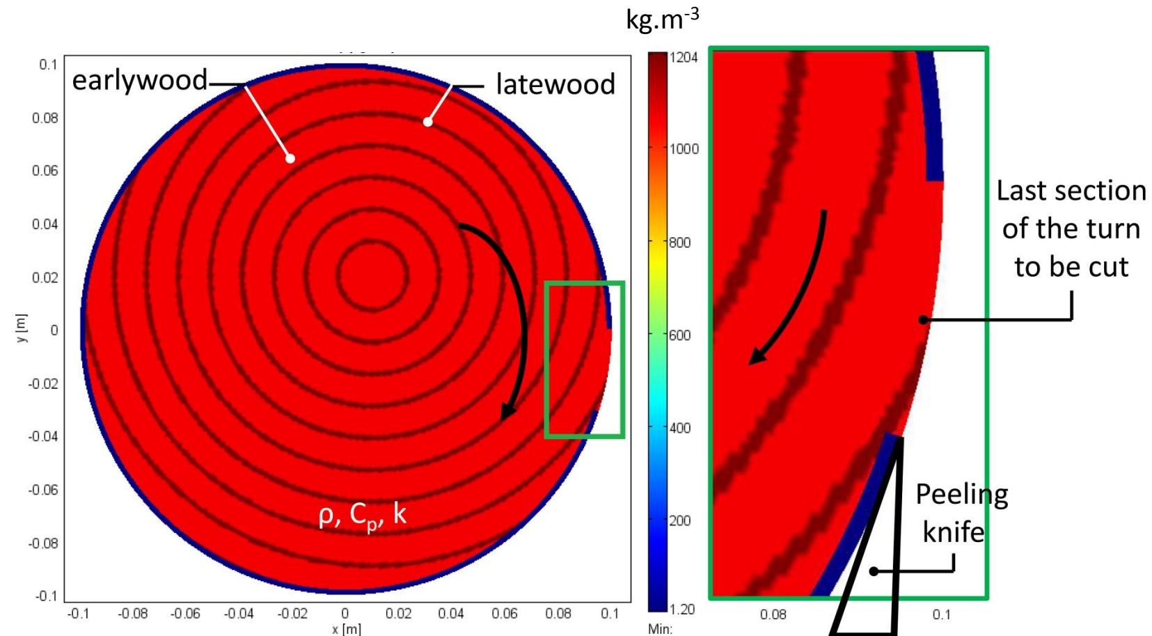
Each Finite Element is parameterized with wood physical properties, taking into account natural defects (knots, rays, off-centered pith)
