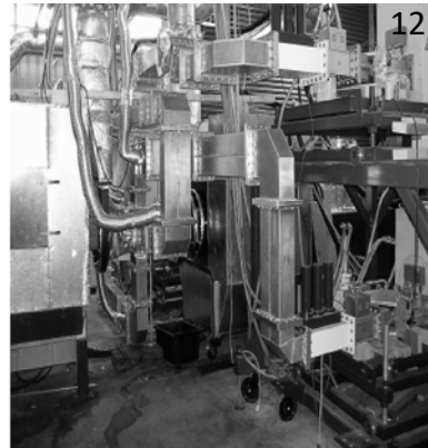
Coaxial cables and waveguides from electric generator to MW applicator.
