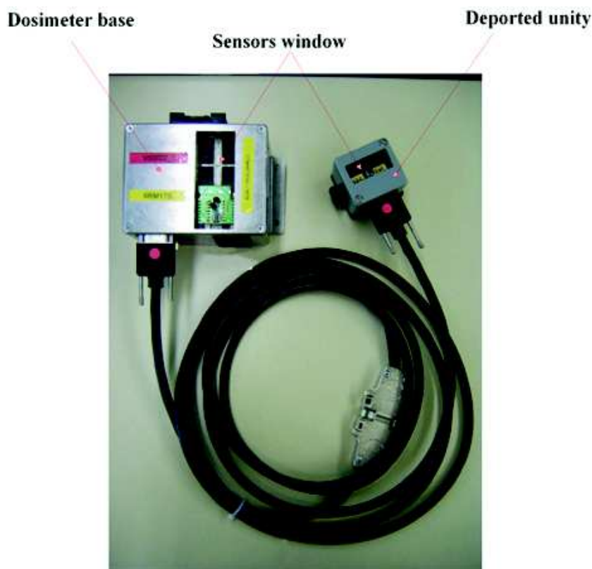
Figure 3-3: Main Board of the RadMon V5 with the deported module.
