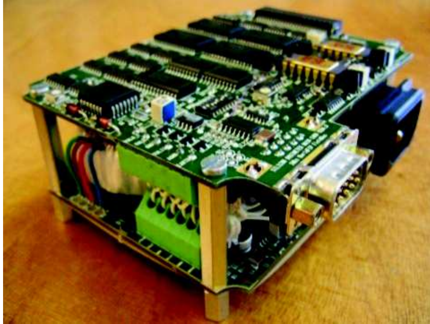
Figure 3-1: RadMon V5 form factor and structure.
