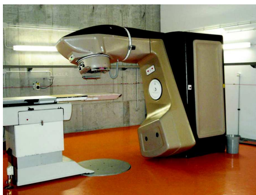
Figure 2-10: AECL Theratron 780 with its rotative arm. The rotation of the arm permits to point the source along the room.
