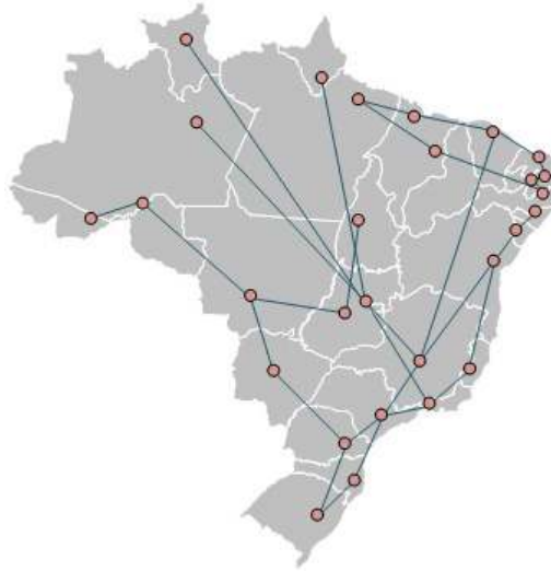
Figure 6.6: The Brazilian Rede Nacional de Ensino e Pesquisa (RNP) real topology, with 31 vertex and 34 edges.
