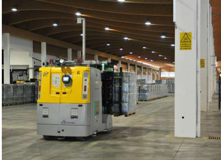
Figure 1: An industrial Ackermann AGV with visible front steering and actuated wheels, its back forklift and a navigation laser scanner at the top of a telescopic pole. Although with slightly different mechanical structure, Dual Drive AGVs have a similar appearance.
