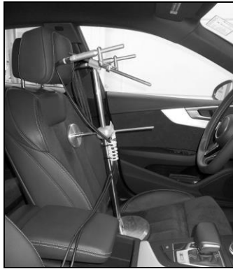
Figure 4: The microphones are positioned on the driver seat inside the car
