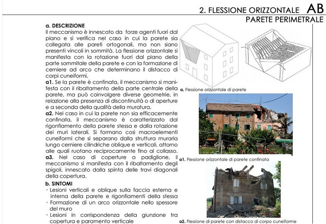
Fig. 7. The abacus/guideline related to the mechanism “2. Horizontal inflection” for “house” matrix type.
