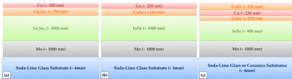
Figure 1. The different precursor layers and sequences used to obtain the absorber material reviewed in this article: (a) first method: deposition in sequence of \text{In}_2\text{Se}_3 – \text{Ga}_2\text{Se}_3 –Cu; (b) second method: deposition in sequence of InSe–GaSe–Cu; (c) third method: deposition in sequence of InSe–GaSe–Cu–GaSe.
