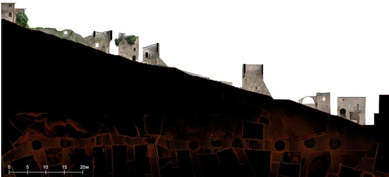
Figure 3. Navelli's main staircase. Orthophoto and laser scanner point cloud.
