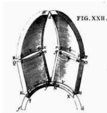
Figure 1. The horizontal thrust of the dome: its “trap” (Poleni 1748). © [rightsholder]. Reproduced by permission of [rightsholder]. Permission to reuse must be obtained from the rightsholder.
