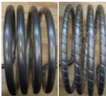
Figure 2. Representative smooth and corrugated helically coiled pipes.
