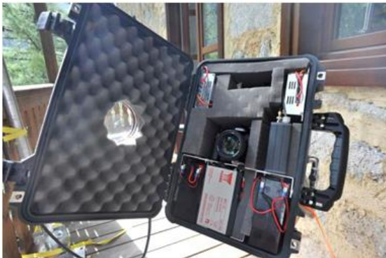
Figure 2: The watertight IP67 box housing all the acquisition and transmit equipment.
