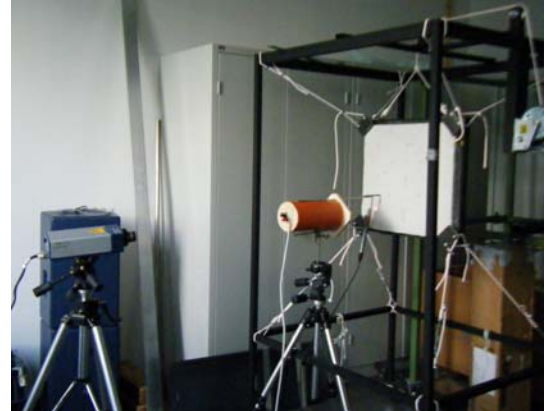
Figure 4. Experimental set-up of the LDV&microphone test.
