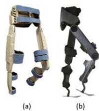
Fig. 2. The Vanderbilt exoskeleton, (a) the prototype of Vanderbilt exoskeleton by Farris et al. [33], (b) the commercialized Indego exoskeleton by Parker Hannifin Corporation [9].
