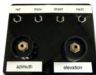
Figure 3. Physical controller designed for the auditory localization test.
