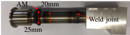
Fig. 9. Heat exchanger trial sample with AM.
