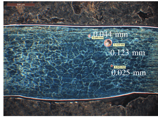
Fig. 10. Metallurgical observations on welding trial of the weld bead with a magnification value of 50x using 52 Amps as back current and 12 Amps as main current.
