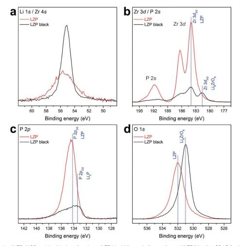
Fig. 7 XPS core levels of LZP-1100 and the black surface layer (LZP black) formed after cycling a Li/LZP/Li cell at 80 °C for 100 h, including (a) Li 1s/Zr 4s, (b) Zr 3d/P 2s, (c) P 2p, and (d) O 1s.
