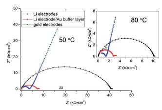
Fig. 4 Impedance plots of LZP-1100 using different electrodes at 50  $^{\circ}\text{C}$  (pellet thickness = 1.5 mm). The inset shows the spectra collected at 80  $^{\circ}\text{C}.$
