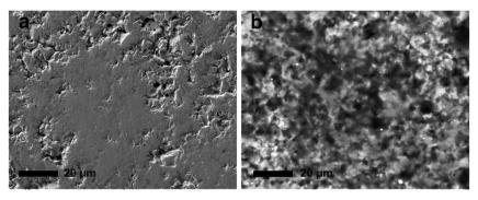
Fig. 5 SEM images of the surface of LZP-1100 pellet before (a) and after (b) galvanostatic cycling at 80 °C for 100 h (40 μA cm<sup>-2</sup>).
