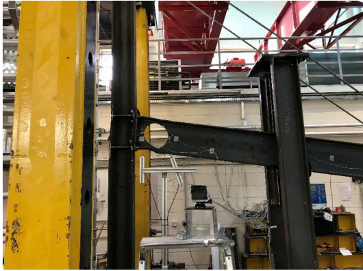
Figure 12 Ultimate failure of RWS_1
