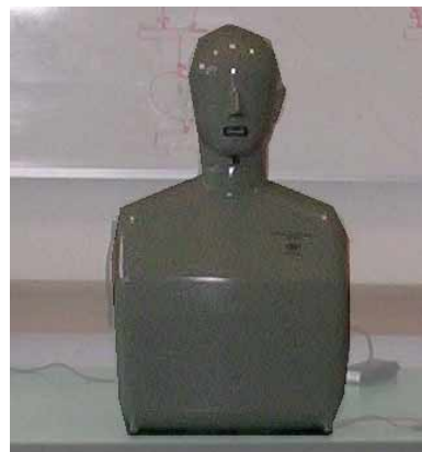
Figure 2 - Brüel & Kjær mouth simulator type 4230.
