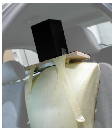
Figure 3 - Small loudspeaker built by Boston mounted on an artificial torso.
