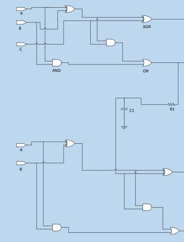
Example of 2-bit Ripple-Carry Adder
